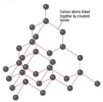
Figure 5 Part of the giant covalent structure of diamond
