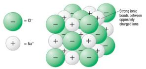
Figure 1 Part of the giant ionic lattice (3-D network) of sodium and chloride ions in sodium chloride
